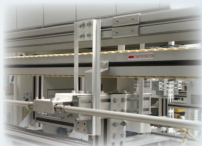
Automated side guide installed at straight section
