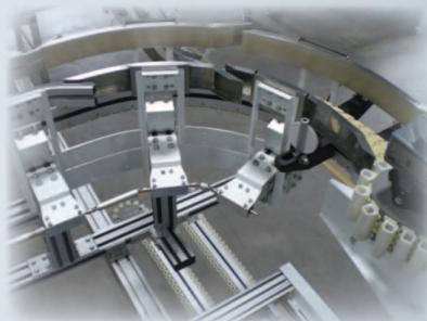
Automated side guide installed at bend section
