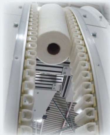
Automated side guide installed at straight section
